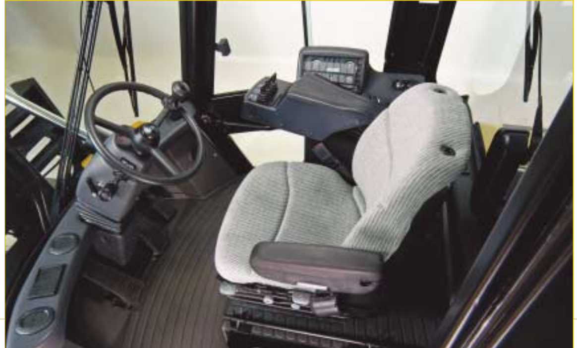
Truck shown with optional enclosed cab, steering spinner knob and full air suspension cloth seat
