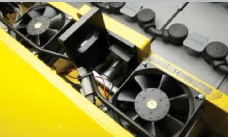
Thermally controlled fans (TCF™) save on battery power.
